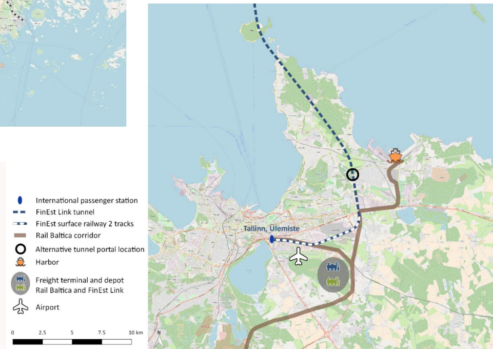
Figure 5.6 Horizontal alignment and facilities in Estonia
